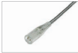
IP64,Clear female connector, 2 cores, UL2468 22AWG L=90/2mm
